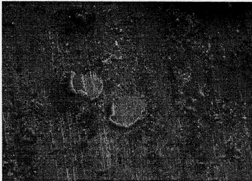
Figure 4: Oxide particles on a mechanically polished non-passivated Type 304L stainless steel surface. Note the areas where the oxide "bubbles" have burst and the bare metal underneath. The white streaks under the top burst bubble probably represents an active stainless steel surface SEM 450X.
