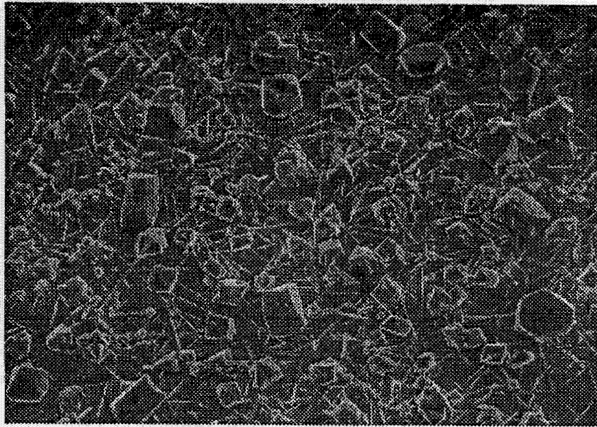
Figure 5: The highly crystalline surface of the gray-black glossy electropolished Type 316L stainless steel tube surface from a steam line. The subsurface crystals appear continuous and the top crystals appear to be joining together. Their crystal form is both octahedral and dodecahedral. This is typical for magnetite. SEM 450X.
