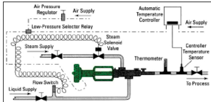
Image 5 - In this configuration, the steam solenoid valve automatically stops steam flow when the liquid flow stops.
