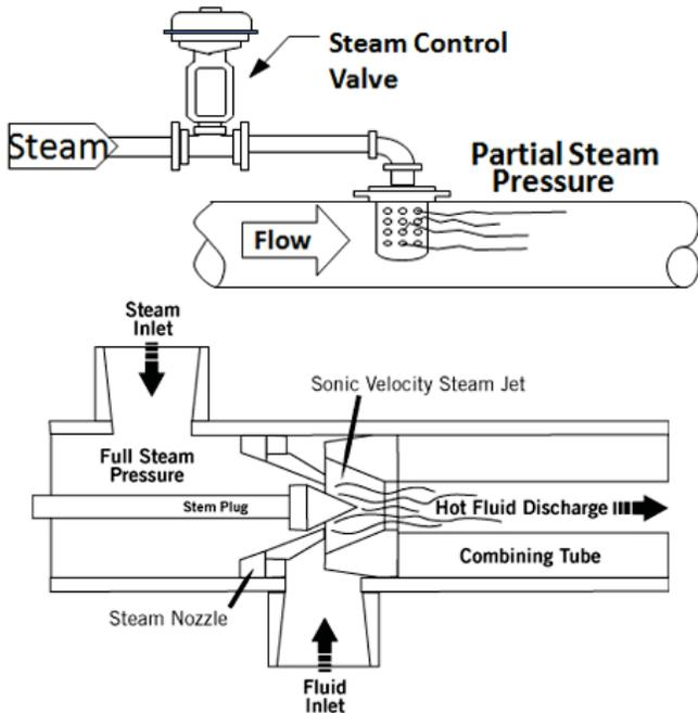
Image 2 - Steam injection may be externally or internally modulated.
