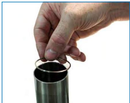
1. ALIGN WELD INSERT WITH THE TUBING
