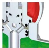
**Closed**Lower valve disc radial seal (RSC seal)
