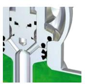
**Movement of lower disc**Lower line closed
