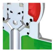
**Closed**Lower valve disc with conical seal
