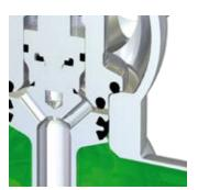
Movement of lower disc Lower line CLOSED Leakage chamber open -> No product loss
