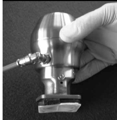
7. For PTFE diaphragm please engage diaphragm bayonet into the compressor slot by applying pressure to the center of the diaphragm. Ensure correct engagement. Continue to apply pressure to the center of the diaphragm and turn through 90°. For rubber diaphragm screw in clockwise direction and avoid over-tightening
