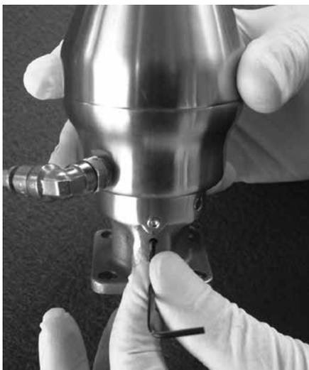
18. Once the spindle adaptor locking screw is undone, remove the spindle adaptor and compressor assembly from actuator bonnet.
