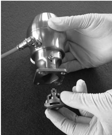
20. Apply Loctite 222 to spindle adaptor locking screw. Insert spindle adaptor and new compressor assembly into actuator bonnet until fully located.
