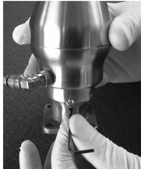
22. Gradually tighten rotation grub screw until actuator bonnet is secure using table two below.
