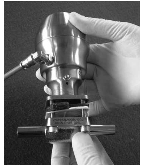
3. Inspect the valve body sealing surfaces for damage.
