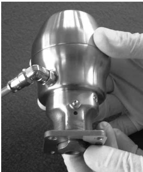
21. Insert Allen Key into actuator bonnet hole and tighten spindle adaptor locking screw fully using table one below.
