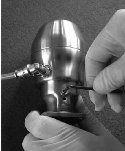
23. Re-attach the actuator to the valve body. Repeat steps 6 to 14.
