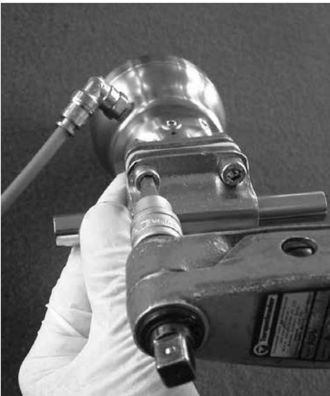
*This ensures that the diaphragm seats correctly before further tightening.*
