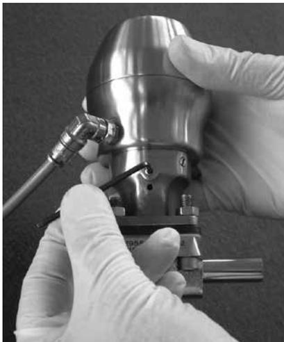
25. Rotate actuator cylinder while actuator is attached to the body, until inlet port is in the required orientation. Rotation feature available on sizes DN15 (0.5 in.) - DN50 (2.00 in.). To facilitate rotation please ensure air supply is "on" for spring closing mode and "off" for spring opening mode.
