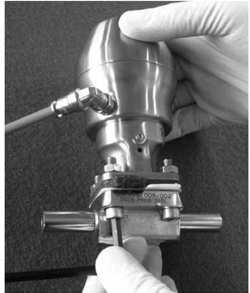
2. Remove the fasteners and the valve actuator.
