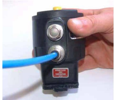
8. Attach the actuator to the valve body; insert the retaining fasteners.
