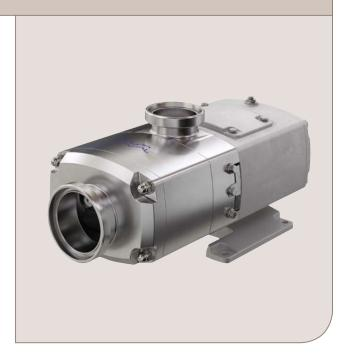
gearcase design optimizes oil circulation to both sets of bearings and the timing gears with an oil sump design. This improves the lubrication effect on both bearings and timing gears, minimizing the energy produced due to friction and thereby reducing heat generation within the pump gearbox.
