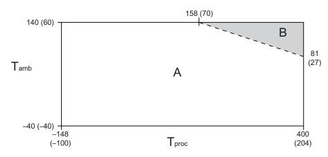
T<sub>amb</sub> = Ambient temperature °F (°C) T<sub>proc</sub> = Process temperature °F (°C) A = All available electronic options B= Extended or remote mount electronics only
