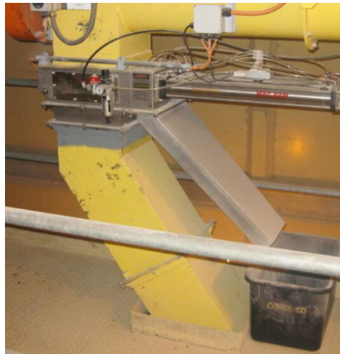
Example of directing the contaminants to a separate container.
