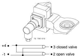
Technical data for female M12 plug - Voltage: 250V AC/DC
