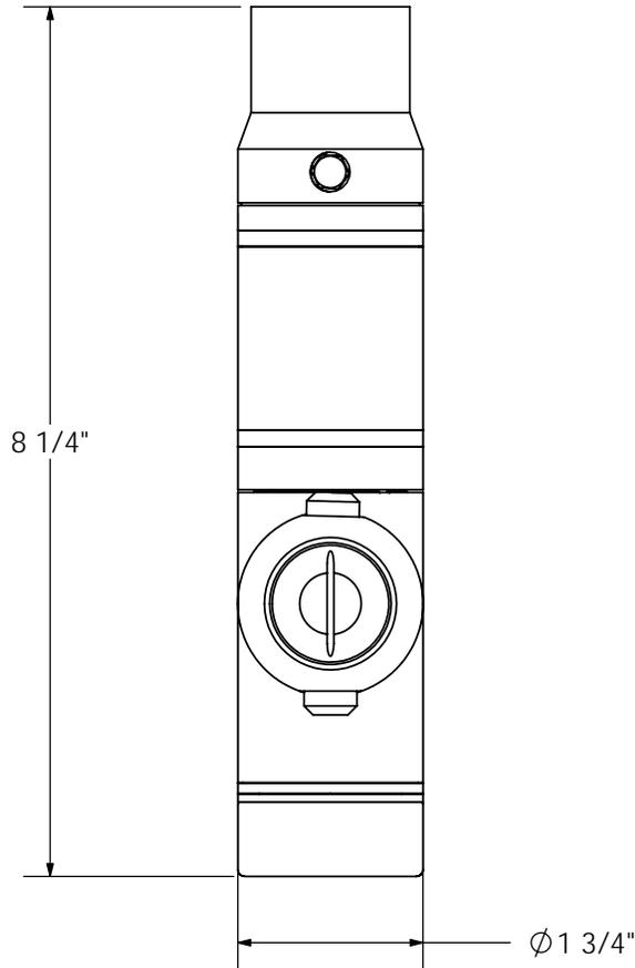
Inlet: 1-1/2" Butt Weld (Shown) or 1" Slip-Joint/Retaining Clip
