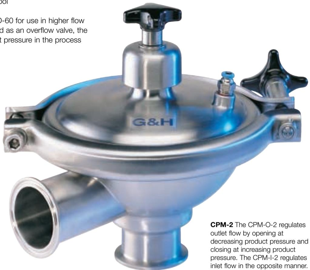
**CPM-2** The CPM-O-2 regulates outlet flow by opening at decreasing product pressure and closing at increasing product pressure. The CPM-I-2 regulates inlet flow in the opposite manner.
