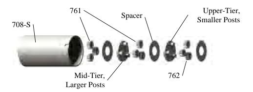
caution. If at any time you do not feel completely comfortable servicing #726, contact Gamajet Cleaning Systems immediately. To eliminate loosing the small internal components, service #726 over a small tray or container. Refer to Section 3.1 for more information.
