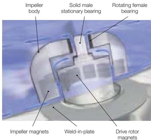
The patented impeller of Alfa Laval magnetic mixers levitates on a magnetic field, which greatly reduces friction and maximizes cleanability.
