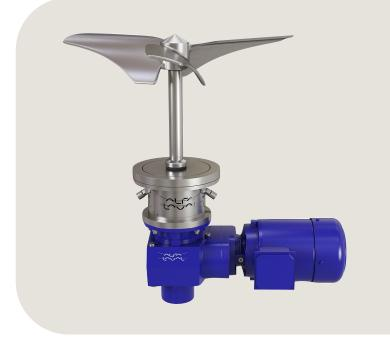
The shaft rotates, turning the EnSaFoil impellers. The impeller movement creates a high flow with low shear due to the highly effective axial pumping effect on the liquid in the tank. This results in effective mixing and blending of the entire contents of the tank.
