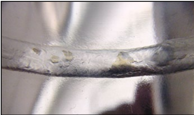
Acceptable weld made in AL-6XN electropolished tubing
