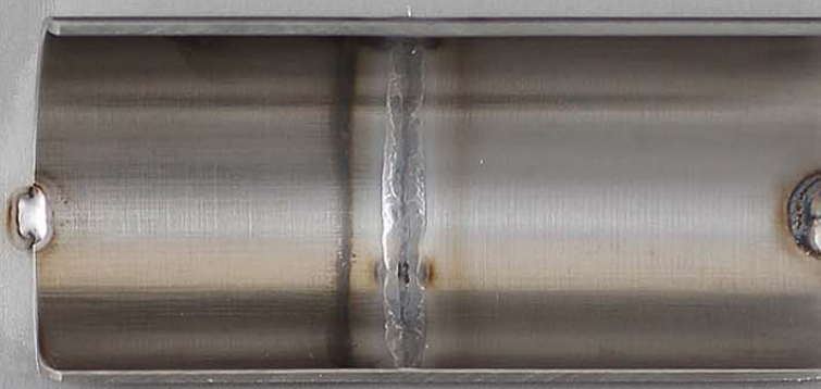
Tack Weld Unconsumed Oxidized Tack Weld Discoloration HAZ
