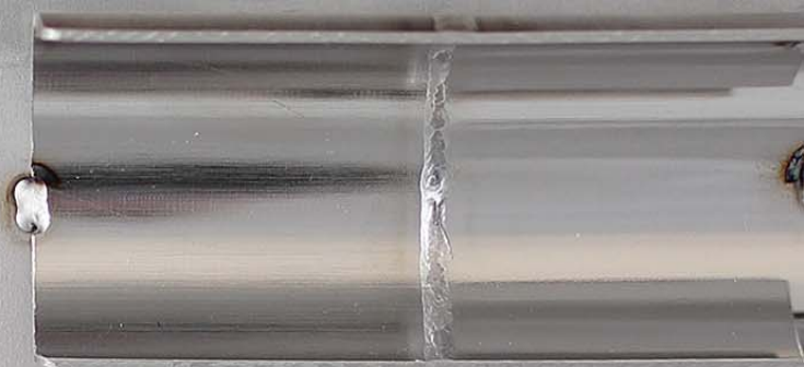
Metal Shaving In Weld Undeburred Tube Cut
