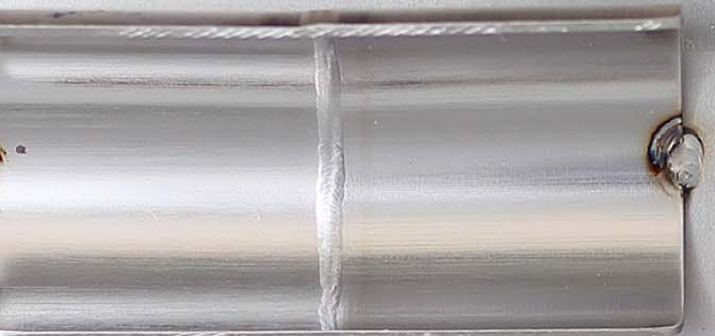
Welded Without Alloy Insert Ring
