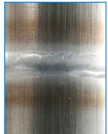
HEAT TINTS REMOVED
