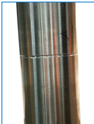
RING WELDED BETWEEN SECTIONS
