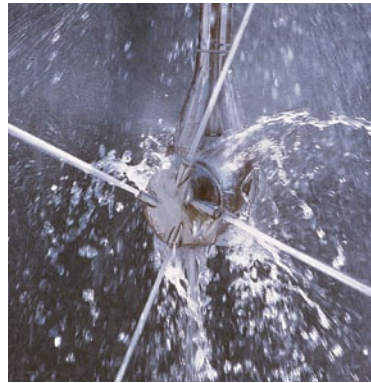
Toffejorg's TJ 20G rotary jet head provides a 360° cleaning pattern inside a vessel.
