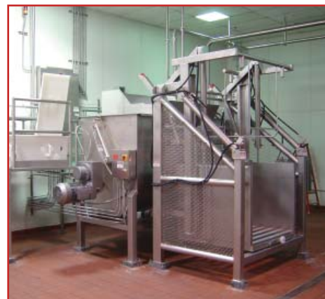
CSI tomato paste dump and blend system, complete with work platform and recipe control system
